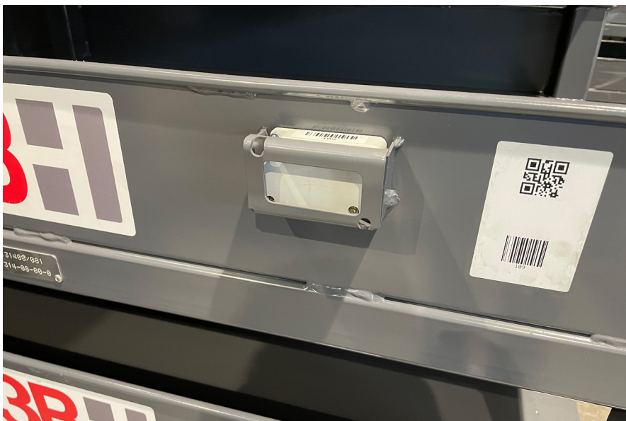
Detail of the Sewio tag attachment to the metallic pallet.
