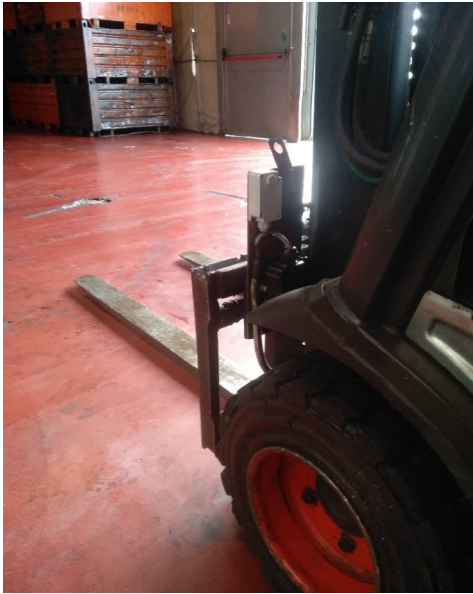
Detail of the tag mounted on the fork of a trolley.
