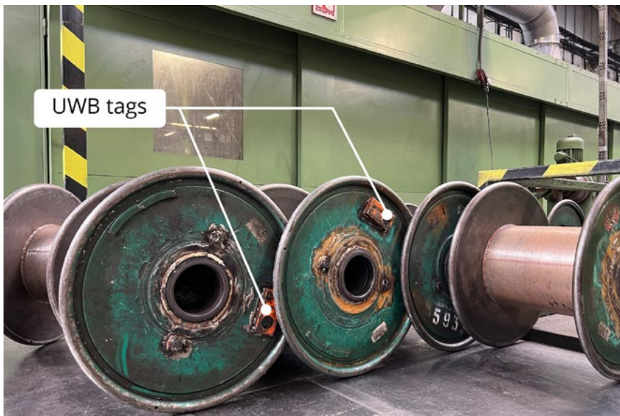
UWB tags mounted on the metallic coils.
